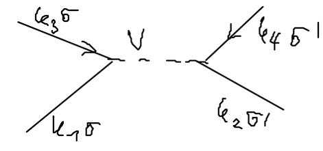
$H_{el-ph} = \sum_{k, q, \sigma} g c_{k+q, \sigma}^{\dagger} c_{k, \sigma} (a_{qn} + a_{-qn}^{\dagger})$
